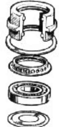
(Right) An "exploded" view of the bottom bevel assembly. When assembling, the interference-fit collar shown here above the lower Oldham coupling is offered up to the shank of the bottom bevel before the coupling is inserted.
