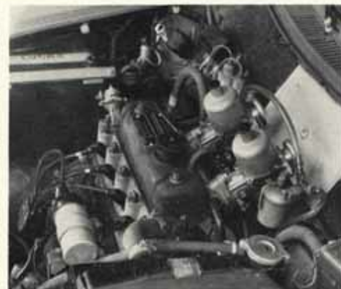
The twin 1¼ in. S.U.'s, light alloy cylinder head and Supertone exhaust system have produced 72 b.h.p. at 6,000 r.p.m. on a compression ratio of 9.5:1. With 1¼ in. S.U.'s fitted, 67 b.h.p. is produced at 5,000 r.p.m. In spite of the absence of air cleaners, there was a creditable absence of roar during acceleration.
