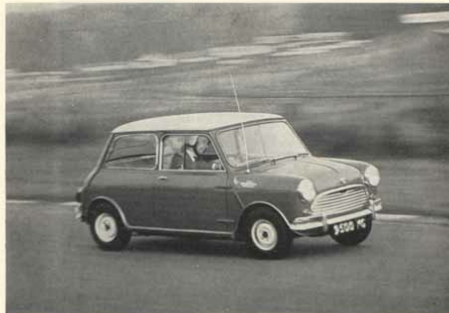
Mini with the lot—even including radio! This fully equipped Speedwell version retains the normal Cooper Mini suspension, apart from different dampers and an anti-roll bar at the rear. But an 82 horsepower engine makes it enormous fun on the track. (John Blunsden testing at Brands Hatch).
