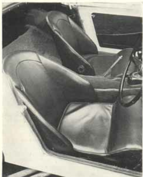
With adjustable squabs, the Restall seats gave good support and were very comfortable. Note the exhaust pipe exit.
