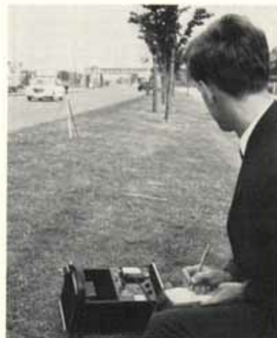
Noise Level Test using Dawes Sound Measuring Equipment.
