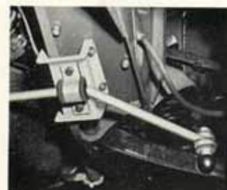
AR.4 anti-roll bar fitted to A.35
