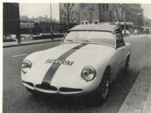
Seen at the Racing Car Show (with hard top in place of soft). Side air intakes of the "Monza" bonnet feed air to oil coolers. Ciblé headlights give adequate illumination.
